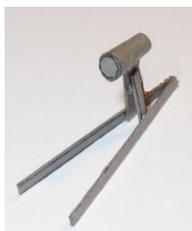
*The acoustic hammer box contained a pneumatic hammer. It was attached to an A-frame at the bow, which could be lowered into the water for sweeping acoustic mines.*
