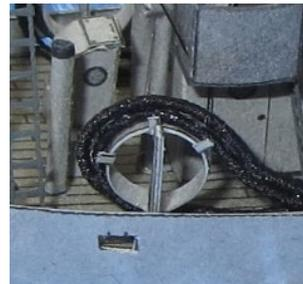
Cable formers: Fold part 20b and cut into small stripes. Glue stripes to part 20a at the markings. Then roll 20a into a ring and glue. Fold the small stripes outwards. Glue the cable guides to supports 20c and then to the bulwarks in line with the fore end of the generator superstructure. Fold cable trunks 20d and cut in stripes.
